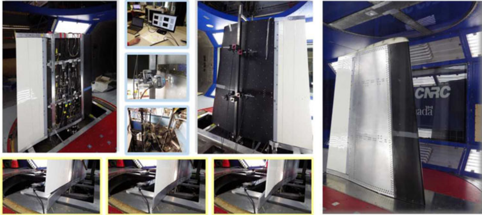
Figure 13. Model installation and calibration in the NRC wind tunnel.
